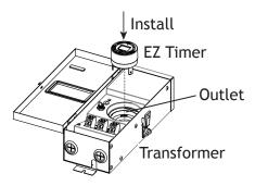
If there is a timer switch module pre-installed in the transformer, remove it before installing the EZ timer.
