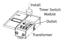
Open the transformer and install the timer switch module into the outlet. This is a circuit completion apparatus that provides an electrical connection.
